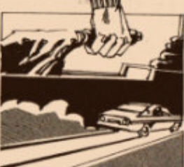
In an emergency use the handbrake, which works on a separate mechanical linkage. It operates the back brakes only, giving you one-third braking power.
