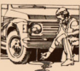
Brakes don't often fail—but when they do it's usually unexpected. The cause is generally a leak in the hydraulic system, so have it inspected regularly.
